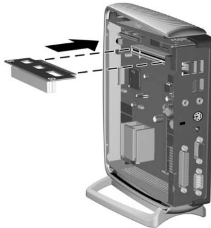
Installing Optional PCI Riser Card
