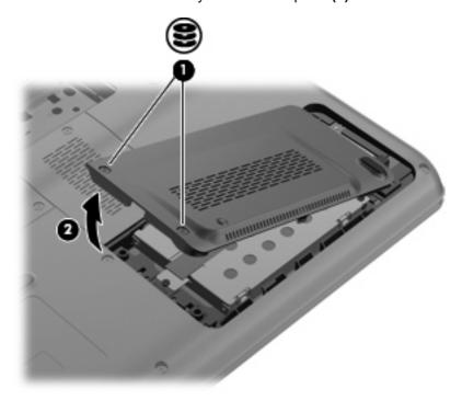
9. Remove the 3 hard drive screws.
