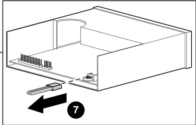
**Identify where the power supply cables are connected before you unplug them.**
