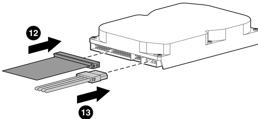
**All connectors are keyed for their intended location and should not require excessive force to plug in.**
