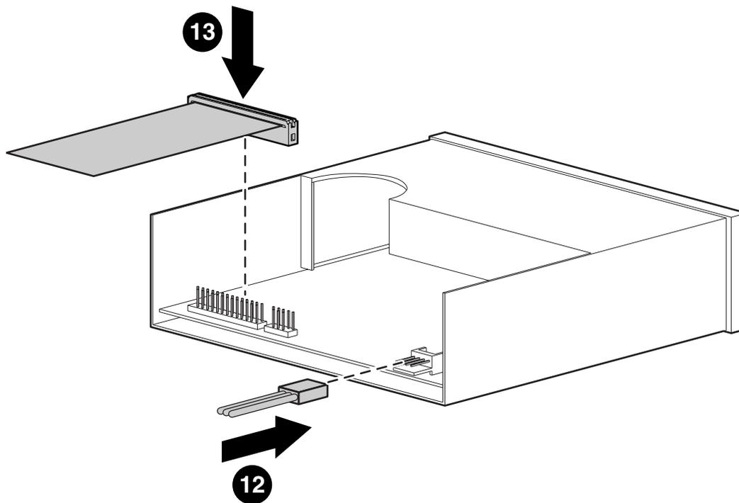
**Note: Use the connector at the end of the cable to connect to the unit. Some cable may have more than one connector; however, only one connector is needed to connect to the unit.**
