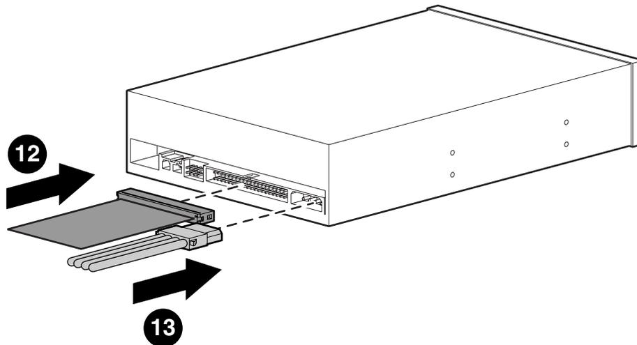
**Note: Use the connector at the end of the cable to connect to the drive. Some cable may have more than one connector; however, only one connector is needed to connect to the drive.**
