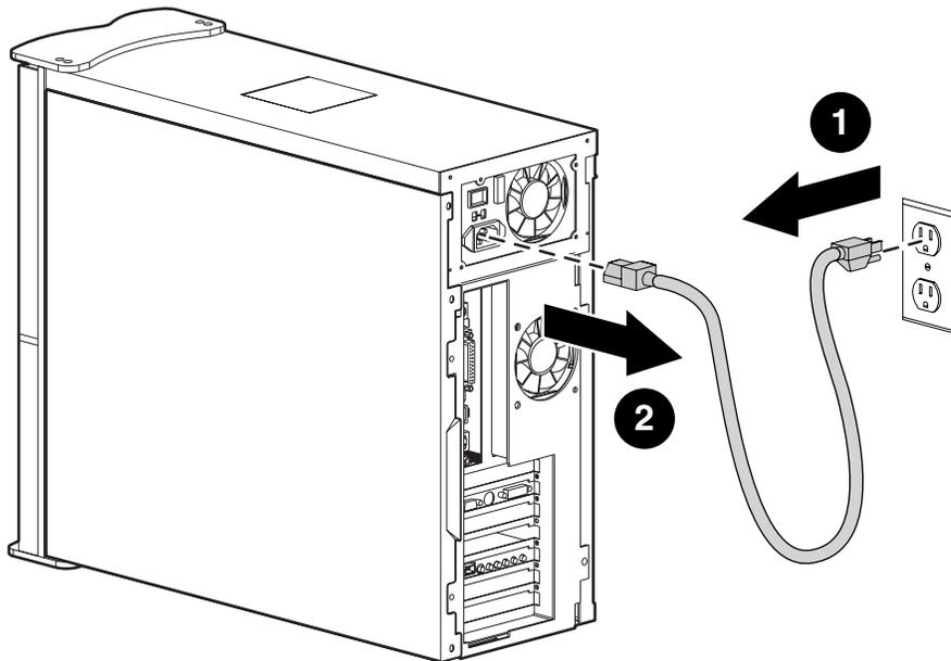
**Warning: Unplug the power cord from the unit and the outlet before replacing any part.**
