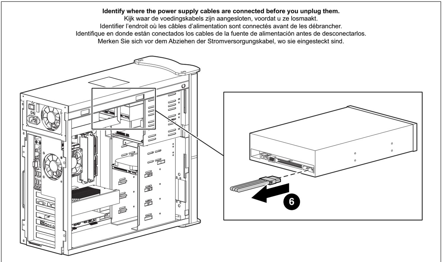
**Identify where the power supply cables are connected before you unplug them.**
