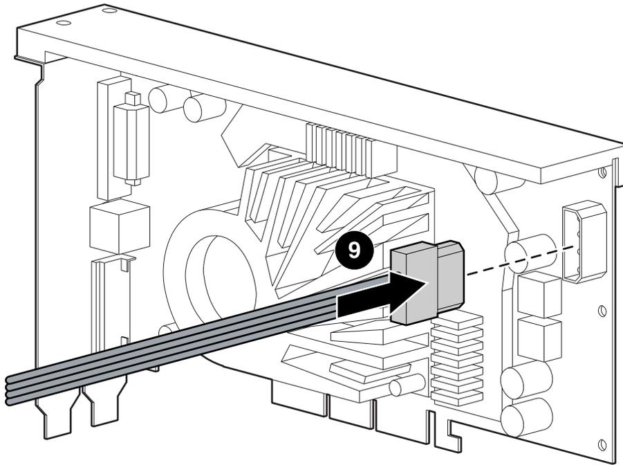
**All connectors are keyed for their intended location and should not require excessive force to plug in.**
