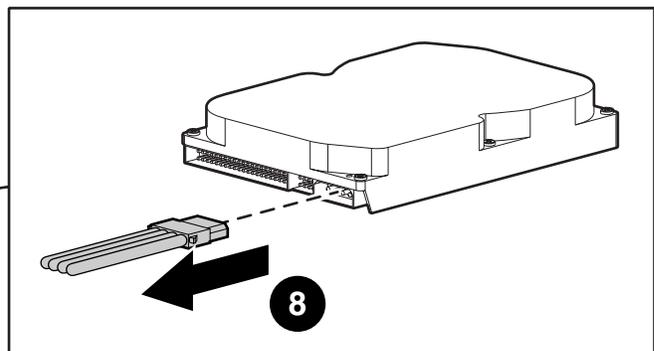
**Identify where the power supply cables are connected before you unplug them.**
