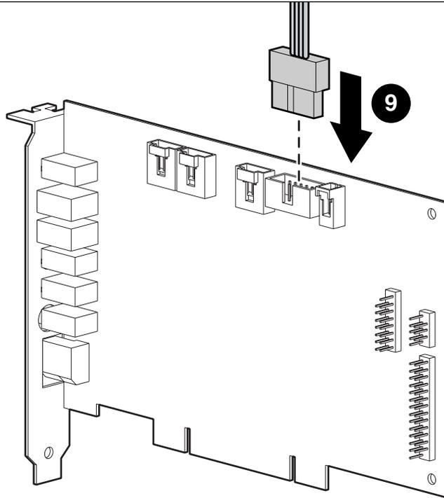
**All connectors are keyed for their intended location and should not require excessive force to plug in.**
