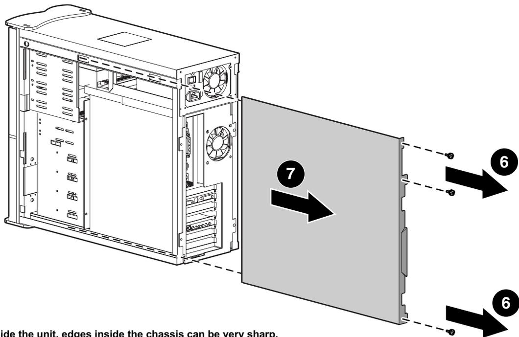
**CAUTION:** When working inside the unit, edges inside the chassis can be very sharp.
