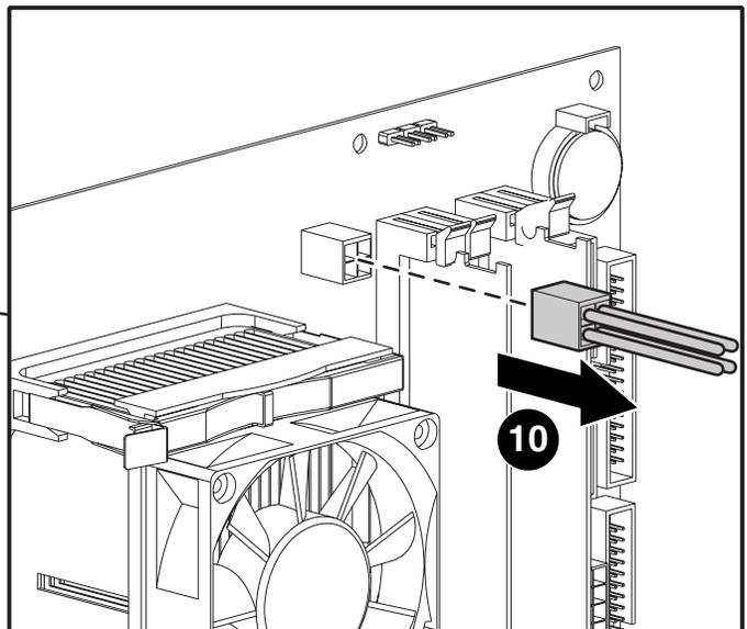
**Some microprocessors may require a power supply cable to be connected to the heatsink fan.**
