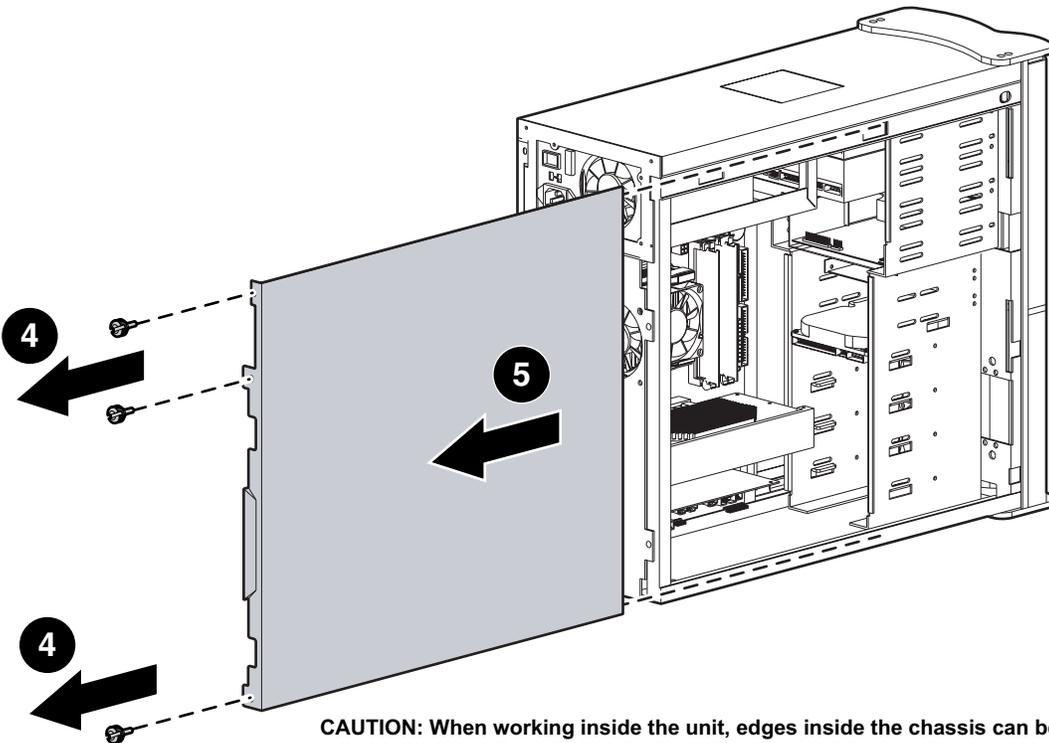
**CAUTION:** When working inside the unit, edges inside the chassis can be very sharp.
