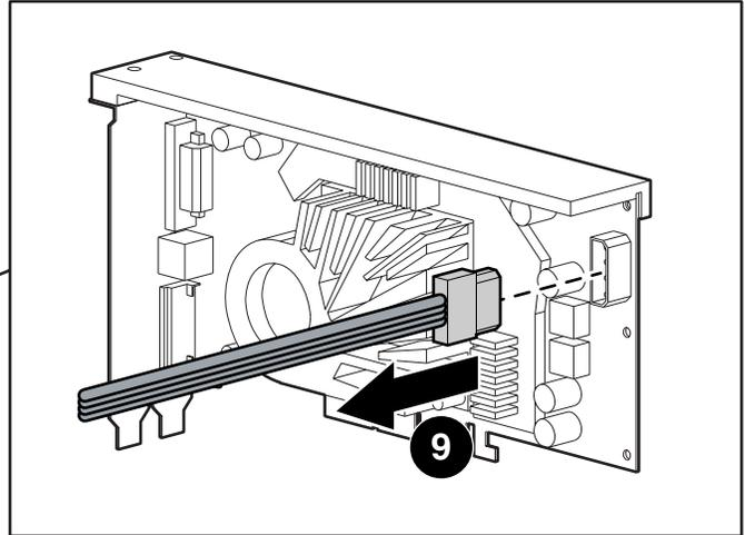
**Identify where the power supply cables are connected before you unplug them.**
