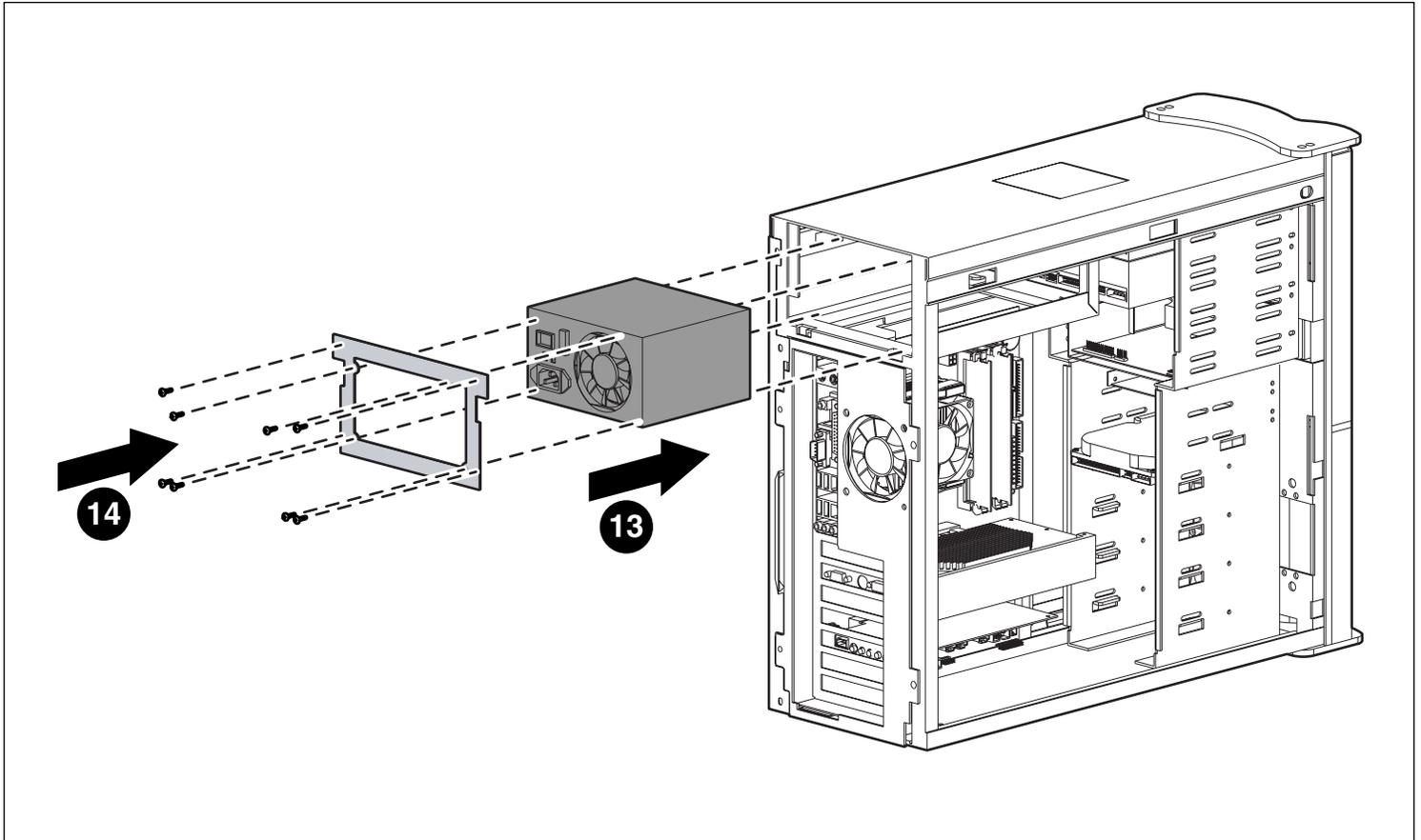
**Installing the power supply into the unit can be done before connecting all the cables to the devices.**
