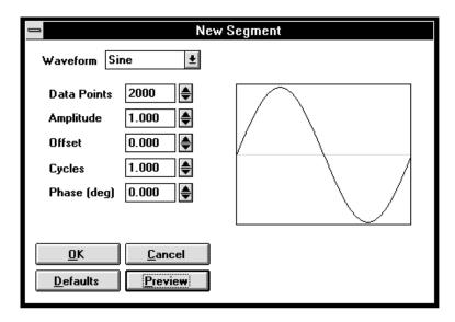
If the selection is made by clicking an icon in the Palette Bar, one segment of the corresponding waveform will be added to the window with default values. If the new waveshape segment causes the total points to exceed 16,000, a warning dialog will appear, informing you that the segment will not be added. Click OK and try a smaller number of points or remove part of the existing waveform.
