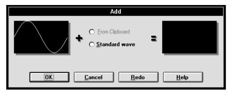
4 The waveform selected for the mathematical operation is displayed in the window on the left. Click the FROM CLIPBOARD button. The waveform previously copied to the Clipboard appears in the middle window and the resulting waveform is displayed on the right.
