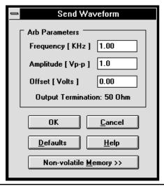
If the I/O | Send Waveform ... menu is not active (gray), HP BenchLink/Arb did not find a function generator on the specified interface. Check that the function generator is properly connected to the computer and turned on. Refer to the section "Configuring the Interface" in Chapter 3 for more information.
