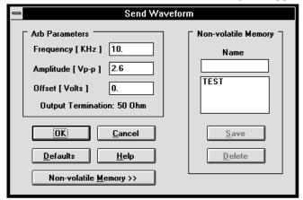
This menu command and icon are only available if a function generator is connected to your PC with an IEEE-488 or RS-232 cable, is displayed in the Instrument list on the Toolbar, and there is waveform data in the waveform edit window.
