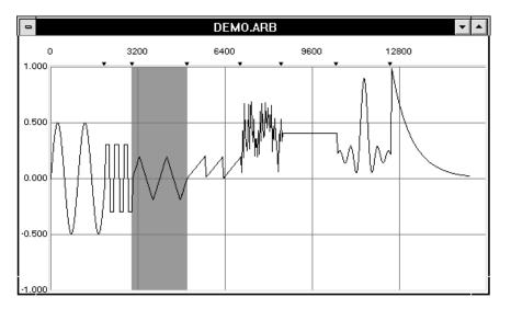
Eight different segments, created from the standard waveshapes, are shown in the figure. The triangle wave segment has been selected and is therefore highlighted. The waveform edit window contains horizontal and vertical gridlines. To change the spacing of the horizontal and vertical grid lines select **View | Grid...** from the Menu Bar.
