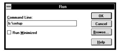
3 During the installation process, the setup program will prompt you for the directory to receive the files. Press ENTER to accept the default installation directory. Type a new drive and directory in the INSTALL TO: text box if needed.
