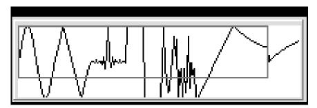
A zoom locator box within the Wave View window shows which part of the overall waveform is currently displayed in the waveform edit window. Move the zoom locator box using a click and drag motion to change the waveform edit window display. Markers are also displayed in the Wave View window (when enabled) to show their location relative to the waveform edit window.
