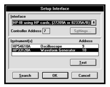
Select the interface type by clicking on the arrow of the INTERFACE drop-down list and clicking on your choice. The controller address or serial port displayed is the IEEE-488 controller address or serial port that HP BenchLink/Arb will use to communicate with your function generator.
