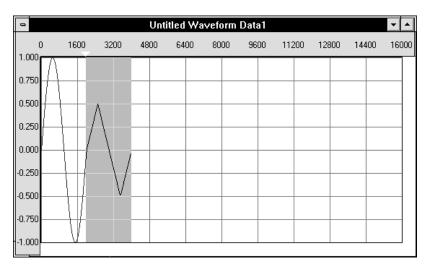
The triangle wave segment amplitude is reduced to 0.5 and the segment is highlighted.
