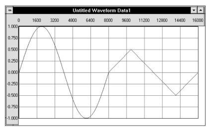
The waveform is expanded to fill all 16,000 data points. The waveform fills the entire window and is now considered arbitrary (you cannot edit the sine wave or triangle wave segments independently).
