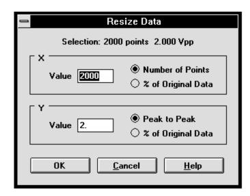
Percentage of Original Data starts at 100%. The size of the waveform data can be changed by specifying the number of points/amplitude peak-to-peak or percentage of the original size. Pressing ENTER for each new value will automatically change the selected data in the waveform edit window. Click OK to complete the resizing process or CANCEL to return the data to its original size.
