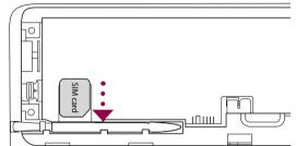
The USIM/SIM card slot is inside the battery compartment.
