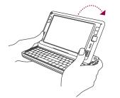
Fold down the touch panel by pressing down on the left and right sides of the panel.
