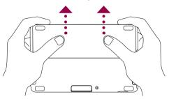
With the bottom side facing up, turn the Mobile Computer so that the battery compartment faces away from you.
