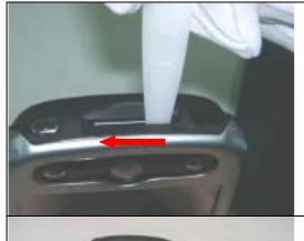
There are three hooks which fix the antenna cover and bezel.
