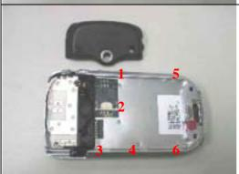
Remove 6 screws which fixed the housing and bezel.
