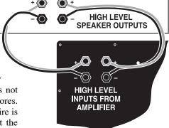
Run the wires from your system's amplifier to the subwoofer's HIGH LEVEL INPUTS. For each channel, run wire from the red (+) outputs on the amplifier to the subwoofer's red (+) inputs, and from the black (-) outputs on the amplifier to the subwoofer's black (-) inputs. Make sure the black amplifier outputs are "true ground." Bridged outputs cannot be used.
