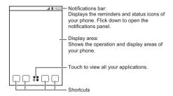
Touch and hold a shortcut until the mobile phone vibrates, you can then drag it to your desired location or move it to the trash. You can also drag an icon from another area of the screen to the shortcut position.
