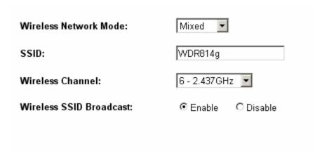
Wireless Network Mode: The ADSL Wireless Router can reach the connection speed of 54Mbps over the 802.11g wireless standard. Also it implements 802.11b for users using early version of wireless. If you have Wireless-G and 802.11b devices in your network, then keep the default setting, Mixed. If you have only Wireless-G devices, select G-Only. If you want to disable wireless networking, select Disable. If you would like to limit your network to only 802.11b devices, then select B-Only.
