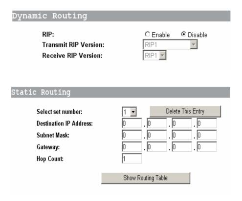
To set up a static route between the Router and another network, select a number from the *Static Routing* drop-down list. (A static route is a pre-determined pathway that network information must travel to reach a specific host or network.) Enter the following data:
