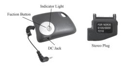
When pulling our from the charger, the blue light flash quickly, the adaptor can not be turned off; only after 1 minute, the blue light flash slowly, the adaptor can be turned off.
