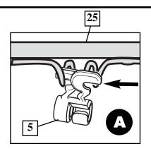
Insert one "arm" of clip into ram as shown. Twist "body" of clip slightly so that second "arm" slides over the top of the first "arm" as shown.
