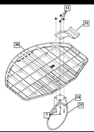
**2.** Attach board assembly to pole.
