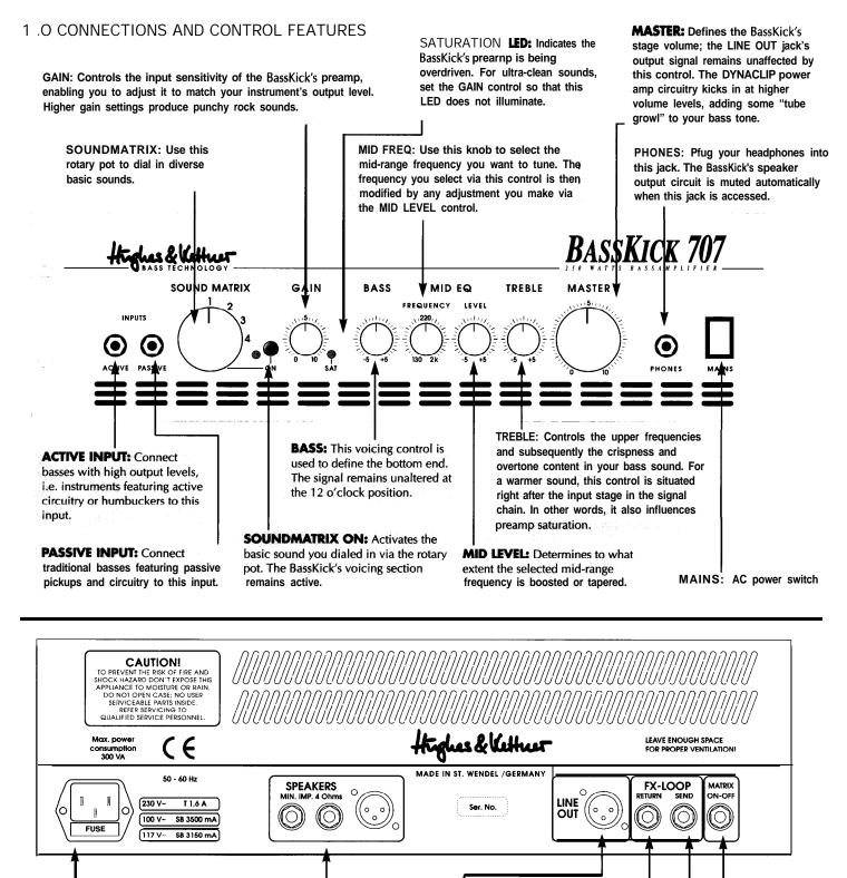
SPEAKERS: Use this output to connect external speakers/cabinets. Ensure the overall impedance is not lower than 4 ohms. For the combo version, you can connect one 8 ohm cabinet, and for the head, a maximum of two 8 ohm speaker cabinets in parallel.
