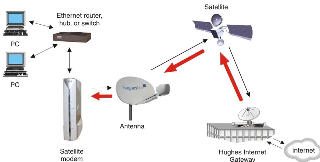
**Figure 3: Multiple-host configuration in an Ethernet wired LAN**
