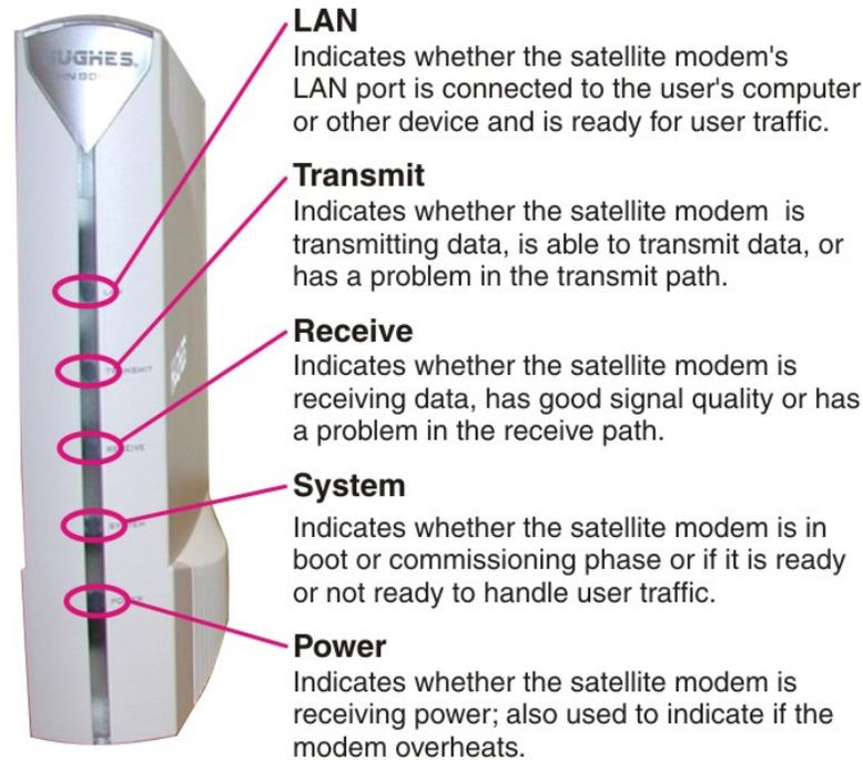
**Figure 22: Front panel LEDs on the HN9000 modem**
