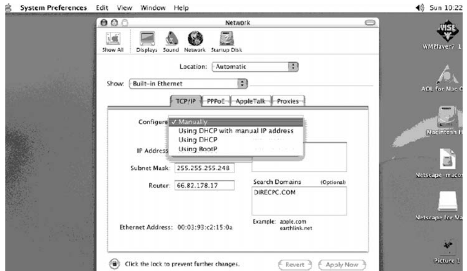
Figure 52: Select Manually from the Configure drop-down list
