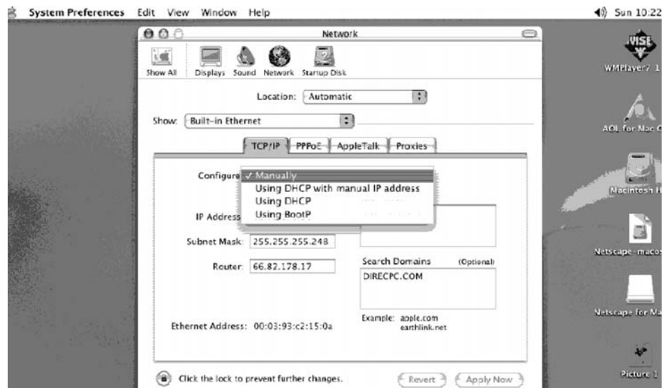
Figure 55: Select Manually from the Configure drop-down list
