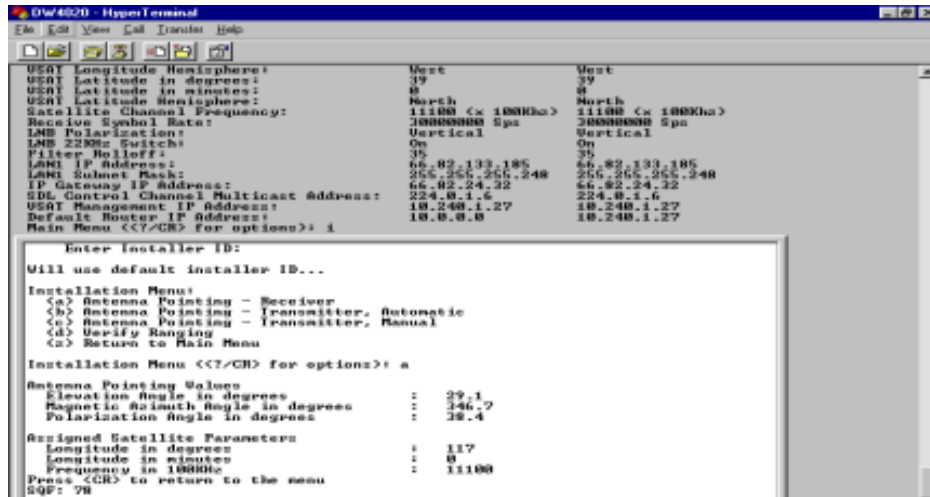
Figure 82: Antenna Pointing - Receiver
