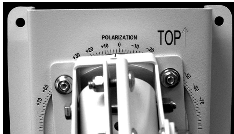
Figure 12: Locating the polarization scale
