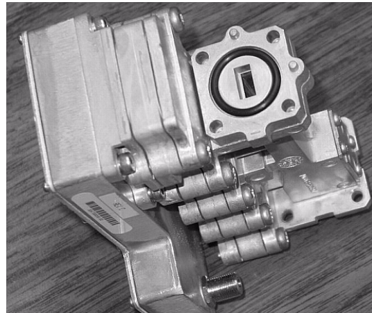
Vertical shim in place (In this photograph, the TRIA has not yet been rotated.)
