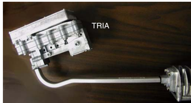
TRIA rotated for vertical polarization
