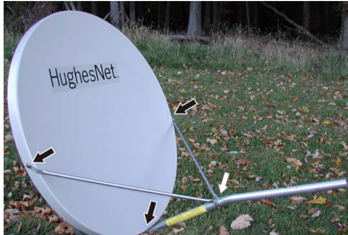
Figure 21: Tightening nuts on feed rods and feed support tube
