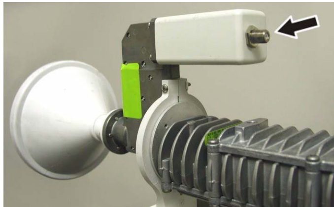
Figure 44: Receive connector – cradle-type radio
