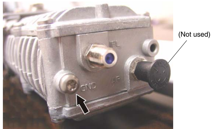
Figure 39: Ground screw on J-type radio assembly (arrow)
