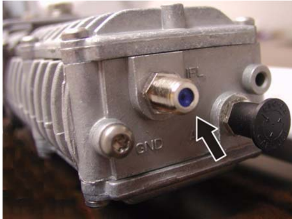
Figure 41: Transmit connector – J-type radio
