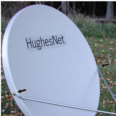
Figure 18: Attaching feed rods to the reflector
