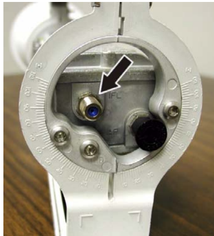
Figure 42: Transmit connector – cradle-type radio
