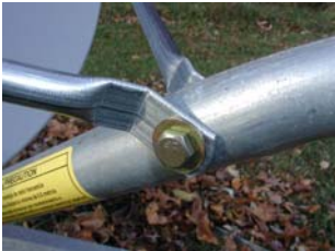
Feed rod ends attached to feed support tube, in front of reflector
