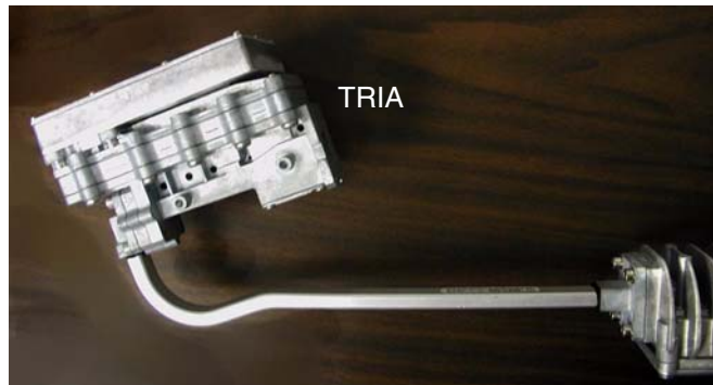
TRIA rotated for vertical polarization
