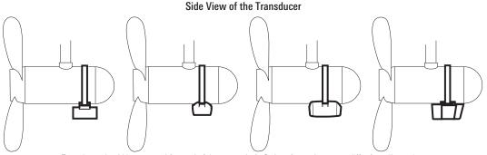
Transducer should be mounted forward of the motor shaft. Styles of transducer may differ from illustration.
