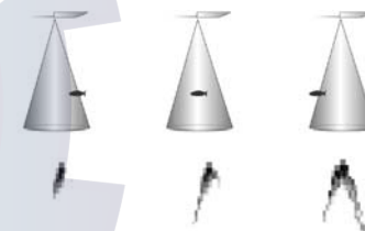
Transducer Cone and Fish Arches
