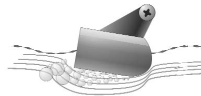
Cavitation that will cause erratic sonar readings
