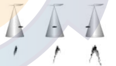
Transducer Cone and Fish Arches
