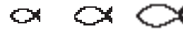
83 kHz, Wide Beam and 455 kHz Side Beam Hollow Fish Symbols (DualBeam PLUS™ and QuadraBeam™ Only)
