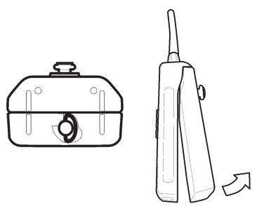
If you are going to use alkaline batteries, remove the alkaline battery compartment cover and install 6 AA alkaline batteries. Re-install the cover to the battery compartment, then secure in place.
