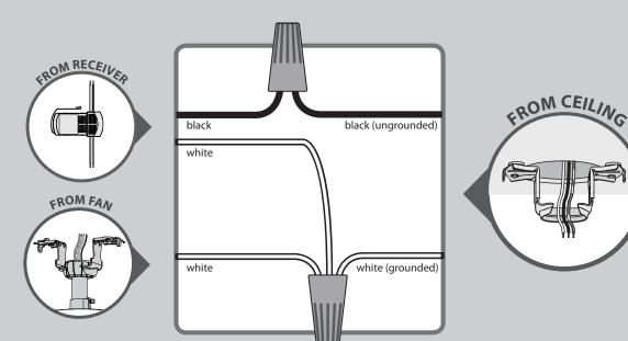
CONNECT WIRES FROM RECEIVER AND FAN TO WIRES FROM OUTLET BOX - Using the orange wire connectors, connect the black wire (ungrounded) from the ceiling to the black wire from the receiver. Connect the white wire (grounded) from the ceiling to both the white wire from the receiver and the white wire from the fan.
