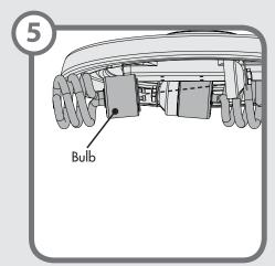
Install a light bulb in each socket.
