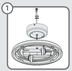
Feed the wires through the center hole in the switch housing, the washer, and the nut. Then install the switch housing by twisting clockwise onto the threaded rod. Install the washer and nut onto threaded rod and tighten securely.
