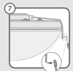
Installing the pull chain pendant -Attach the pull chain pendant to the end of the short chains coming from the switch housing and the light kit.
