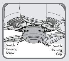
If your fan's switch housing cap resembles this one, remove the whole switch housing by removing the switch housing screws with a Phillips head screwdriver. Remove the two cap screws from the inside of the switch housing. Reinstall the switch housing. Tighten the switch housing screws. Then follow the **TYPE-A ASSEMBLY INSTRUCTIONS** on pages 4-5.
