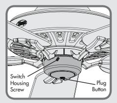
If your fan's switch housing cap resembles this one, remove the whole switch housing by removing the switch housing screws with a Phillips head screwdriver. Remove the plug button. Then follow the **TYPE-B ASSEMBLY INSTRUCTIONS** on pages 6-7.
