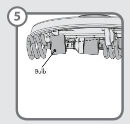
Install a light bulb in each socket.
