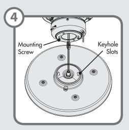
Lift the light kit up to meet the lower switch housing. Wrap keyhole slots around the screws and twist counterclockwise. Tighten screws.
