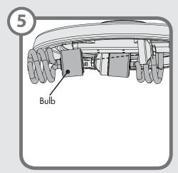
Install a light bulb in each socket.
