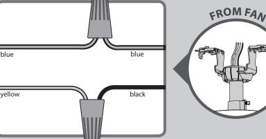
CONNECT WIRES FROM RECEIVER TO FAN - Using the orange wire connectors, connect the blue wire from the receiver to the blue wire (or possibly black with white stripe wire) from the fan. Connect the yellow wire from the receiver to the black wire from the fan.
