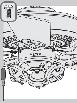
Install the third switch housing screw.
