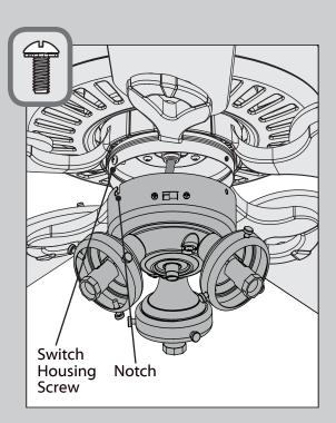
Align the notches in the sides of the lower switch housing with the screws on the upper switch housing. Twist the lower switch housing clockwise to lock into place.
