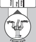
Turn the splices upward and push them carefully back through the hanger bracket into the outlet box. Spread the wires apart, with the grounded wires on one side of the outlet box and the ungrounded wires on the other side of the outlet box.
