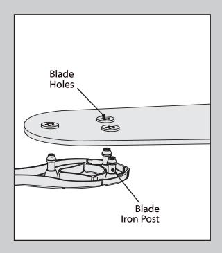
Align the three holes in the blade with the three blade iron posts. Squeeze the blade and the blade post together.
