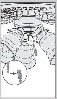
Connect a pull chain pendant to each of the short chains coming from the switch housing.
