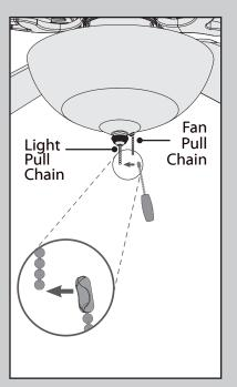
Connect the appropriate pull chain pendant to each of the short chains coming from the finial and finial cap. The fan pull chain controls the speed: from high to off. The light pull chain controls the light fixture: on and off.
