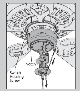
Align the notches in the sides of the lower switch housing with the upper switch housing screws. Lift the lower switch housing. Twist the lower switch housing clockwise to lock into place. Then thread the fan pull chain through the hole in the light kit.
