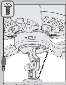
Install the third switch housing screw.
