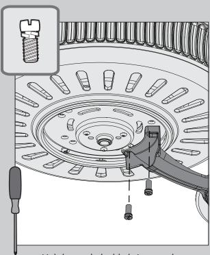
Lightly attach the blade irons to the motor with screws found in the ☒ hardware bag, then securely tighten after both screws are attached.
