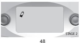
Low battery warning – indicates two stages of battery power shortage.
