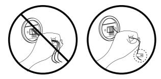
NOTICE! Do not disconnect the wires from the existing thermostat before reading these instructions. The wires must be labeled prior to removal to ensure proper reconnection.
