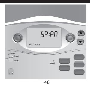
5. Span setting mode – allows you to adjust the system ON/OFF cycle rate. The default setting is 2 (the system cycles ON or OFF when the temperature is within 1<sup>o</sup> F (0.5<sup>o</sup> C) above and below the set temperature.) The span setting can be adjusted if your system is cycling too fast or too slowly.
