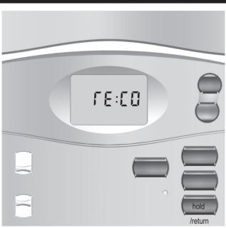
5. Auto recovery – allows heating and cooling systems to gradually recover from an energy-saving setpoint temperature to a comfort setpoint temperature. Auto recovery calculates the time needed to adjust the temperature to the next program setting. When the thermostat is in Auto Recovery mode, the display will flash alternating messages of RECO and the time. Auto Recovery can be disabled by sliding the recovery switch on the back of the circuit board to the disable position.
