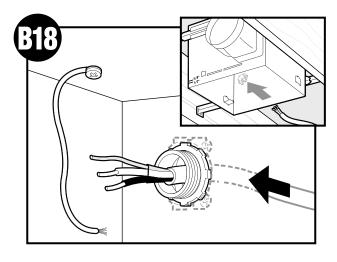
Pull wires through the strain relief.
