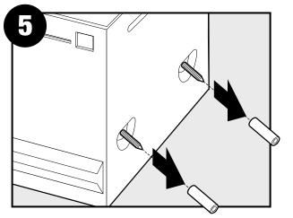
Remove the pre-loaded screw tip covers.
