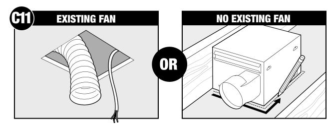
Remove an existing fan and check to make sure the opening is large enough to accommodate the new motor housing (9" x 9.75").
