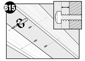
Insert screws, leaving space between the screw head and the joist. Screws are not provided.
