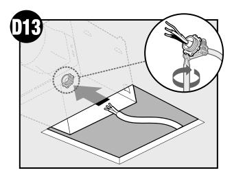
Pull wires through strain relief.
