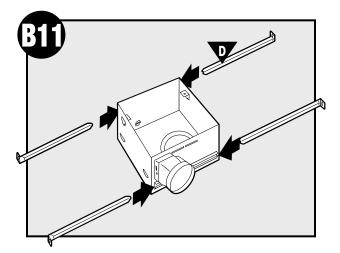
Slide the mounting rails into brackets.
