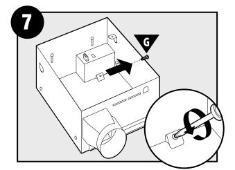
Remove the wiring cover screw.
