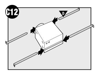
Slide the mounting rails into brackets.
