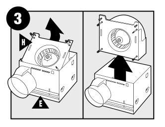
Remove the motor/blower from the housing.
