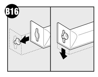
Attach the rails onto the screws.
