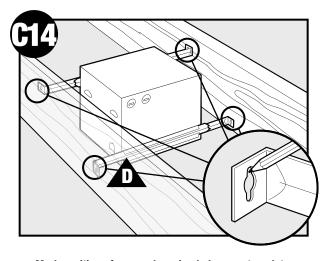
Mark position of screws by using holes as a template.
