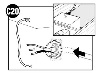
Pull wires through the strain relief.
