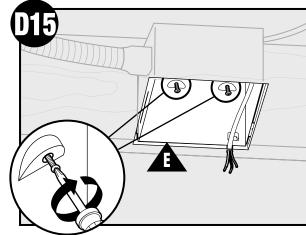
Screw pre-loaded screws into joist or framing.
