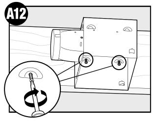
Screw pre-loaded screws into joist or framing.
