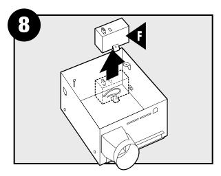
Remove the wiring cover.
