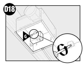
Tighten the wiring cover plate screw.
