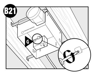
Tighten the wiring cover plate screw.
