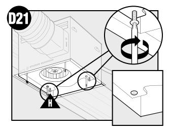
Secure the motor by tightening the 2 screws.
