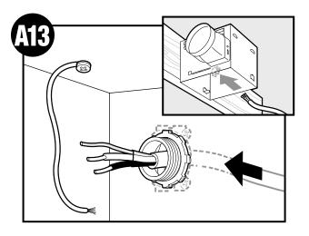
Pull wires through the strain relief.
