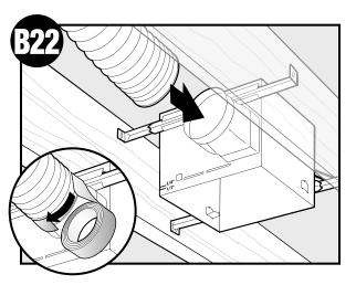
Connect 4" duct and vent to the outside. Tape joints.
