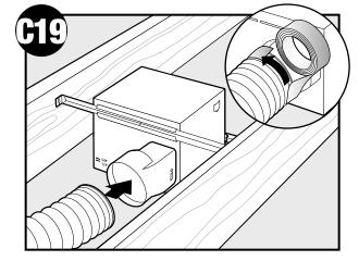
Connect 4" duct and vent to the outside. Tape joints.
