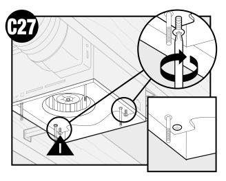
Secure the motor by tightening the 2 screws.
