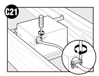
Tighten the strain relief screws.
