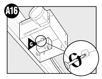
Tighten the wiring cover plate screw.
