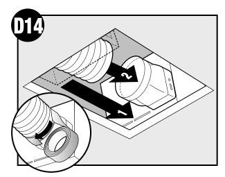
Attach existing ducting to duct connector. Tape joints.
