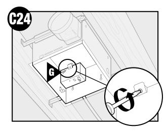
Tighten the wiring cover plate screw.
