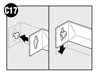
Attach the rails onto the screws.
