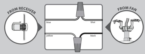
CONNECT WIRES FROM RECEIVER TO FAN - Using the orange wire connectors, connect the blue wire from the receiver to the blue wire (or possibly black with white stripe wire) from the fan. Connect the yellow wire from the receiver to the black wire from the fan.
