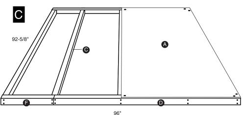
D: Position the other 48" x 92-5/8" Floor Panel A flush against first panel and flush to edges of Floor Frame. Secure panel with two 2" nails at outside corners and one 2" nail at each of other corners.
