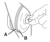
The shaft can be locked using a screwdriver, steel pin or the like. This is slid in as far as possible. The blade is tightened clockwise.
