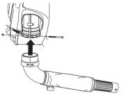
Also pay attention to the stops located on the pipe bend and the fan's outlet pipe. Ensure that the stop on the pipe bend comes in front of the stop on the outlet pipe.
