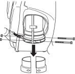
Place these on the pipe bend so that the guide on the wear ring halves aligns with the slot on the pipe bend.
