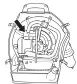
The muffler is equipped with a special spark arrestor mesh. The spark arrestor mesh should be cleaned once a month. This is best done with a wire brush.
