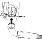
• Also pay attention to the stops located on the pipe bend and the fan's outlet pipe. Ensure that the stop on the pipe bend comes in front of the stop on the outlet pipe.
