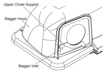
3. Secure upper chute support to hood with hex bolts, washers and nyloc nuts.
