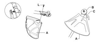
**142R:** Fit the guard (A) to the gear housing using the support plate (M) and two screws (L). CAUTION! Ensure that the guard extension is fitted.
