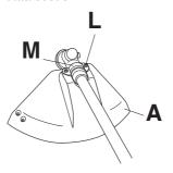
**143R:** Hook the blade guard/combination guard (A) onto the fitting on the shaft and secure with the bolt. CAUTION! Ensure that the guard extension is removed. Use the recommended blade guard. See the Technical data section.
