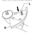
**133R:** Hook the blade guard/combination guard (A) onto the fitting on the shaft and secure with the bolt (L).
