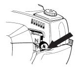
Choke: Set the choke control in the choke position.
