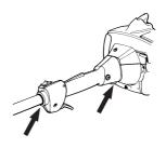
Check that the vibration damping element is undamaged and securely attached.
