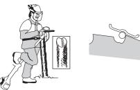
The filing angle is 15°. File alternate teeth to the right and those in between to the left. If the blade has been heavily pitted by stones it may be necessary to dress the top edges of the teeth with a flat file, in exceptional cases. If so, this should be done before filing with a round file. The top edges must be filed down by the same amount for all the teeth.
