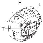
The L and H-jets are used to adjust the supply of fuel to match the rate that air is admitted, which is controlled with the throttle. If they are screwed clockwise the air/fuel ratio becomes leaner (less fuel) and if they are turned anti-clockwise the ratio becomes richer (more fuel). A lean mixture gives a higher engine speed and a rich mixture gives a lower engine speed.
