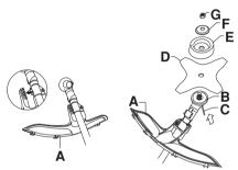
Hook the blade guard/combination guard (A) onto the fitting on the shaft and secure with the bolt. CAUTION! Ensure that the guard extension is removed.
