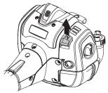
Remove the air filter cover and take out the filter. Wash it clean in warm, soapy water. Clean also the inside of the filter cover by using air or a brush. Ensure that the filter is dry before refitting it.
