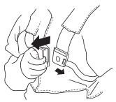
Check that the harness straps are correctly positioned. Once the harness and machine have been adjusted, check that the harness guick release works correctly.
