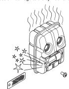
CAUTION! Never use a machine with a defective muffler.
