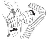
The guide roller is pressed into the knob. In order to loosen the guide roller, you need to continue turning the knob until it loosens completely.
