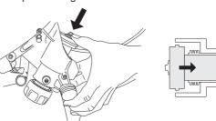
Lubricate the guide roller's sleeve using grease. Fit the grease gun on the grease nipples (A) and pump in grease until clean grease emerges from the overflow hole (B).
