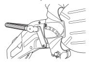
Remove the three screws holding the support roller guard using a 6 mm hex key and lift off the cover.
