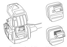
Some mufflers are equipped with a special spark arrestor screen. If your machine has this type of muffler, you
