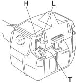
The L and H-jets are used to adjust the supply of fuel
