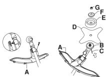
Hook the blade guard/combination guard (A) onto the fitting on the shaft and secure with the bolt.
