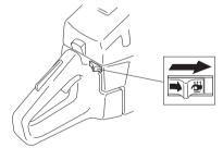
When the switch is pushed to the right, the heat is switched on. When the switch is pushed to the left, the heat is switched off.
