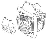
The filter can be cleaned more thoroughly by washing it in water and detergent.
