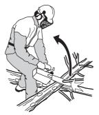
Have control over the workpiece. If the pieces you intend to cut are small and light, they can jam in the saw chain and be thrown towards you. Even if this does not need to be a danger, you may be surprised and lose control of the saw. Never saw stacked logs or branches without first separating them. Only saw one log or one piece at a time. Remove the cut pieces to keep your working area safe.
