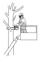
8 Take great care when you cut with the top edge of the bar, i.e. when cutting from the underside of the object. This is known as cutting with a pushing chain. The chain tries to push the chain saw back towards the user. If the saw chain is jamming, the saw may be pushed back at you.
