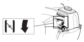
Hold the body of the machine on the ground using your left hand (CAUTION! Not with your foot!). Grip the starter handle, slowly pull out the cord with your right hand until you feel some resistance (the starter pawls grip), now quickly and powerfully pull the cord. Never wrap the starter cord around your hand
