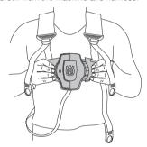
Check that the harness straps are correctly positioned. Once the harness and machine have been adjusted, check that the harness guick release works correctly.
