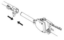
Before using the unit, tighten the knob securely.
