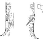
Next make the bottom cut so that it finishes exactly at the end of the top cut.
