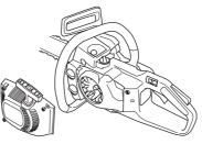
Pull out the cord approx. 30 cm (12 inches) and hook it into the notch in the rim of the pulley. Release the recoil spring by letting the pulley rotate slowly backwards.
