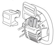
The filter can be cleaned more thoroughly by washing it in water and detergent.
