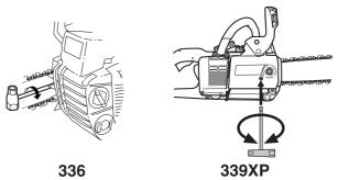
The chain is correctly tensioned when it does not sag from the underside of the bar, but can still be turned easily by hand. Hold up the bar tip and tighten the bar nuts with the combination spanner.
