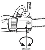
• Use the combination spanner to tighten the bar nuts while lifting the tip of the bar at the same time. Check that you can pull the chain round freely by hand and that it does not sag from the underside of the bar.
