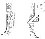
The directional cuts should run 1/4 of the diameter through the trunk and the angle between the top cut and bottom cut should be  $45^{\circ}$ .
