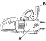
The brake is applied when the front hand guard (B) is pushed forwards.
