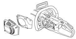
Clean the cooling system with a brush once a week, more often in demanding conditions. A dirty or blocked cooling system results in the machine overheating which causes damage to the piston and cylinder.
